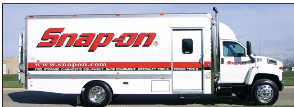
This Chevrolet C7500 above is shown with a 22-foot US Truck riveted body
